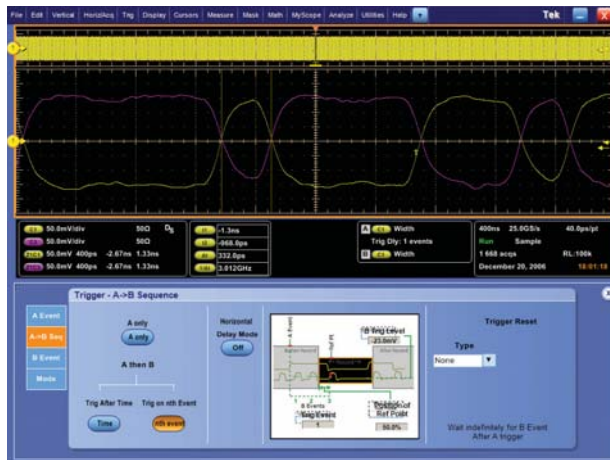
Figure 6 You use the AB-sequence trigger, with the A event set to trigger on the 0000 sequence before the lone bit and the B event set to trigger on the 0000 sequence after the lone bit. With a stable trigger on the lone-bit pattern, you can now perform the jitter and eye analysis on as many consecutive triggers as necessary.
