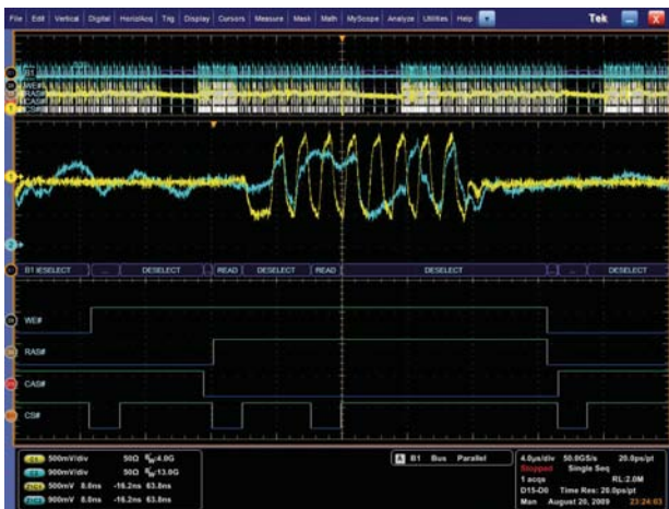
Figure 8 You use pattern-symbol files when a group of signals define a logical state, such as the SDRAM-command group.
