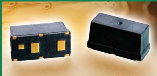
Figure A The RTP device offers simplified thermal protection in an SMD package. It provides protection due to copper-loss heating in resistive faults, such as a failed FET in resistive mode, in which overcurrent is not a factor.
