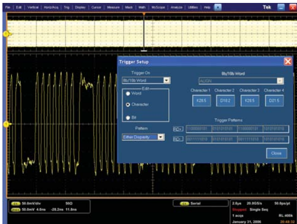
Figure 5 This SERDES-based trigger can respond to disparity and character errors in real time.
