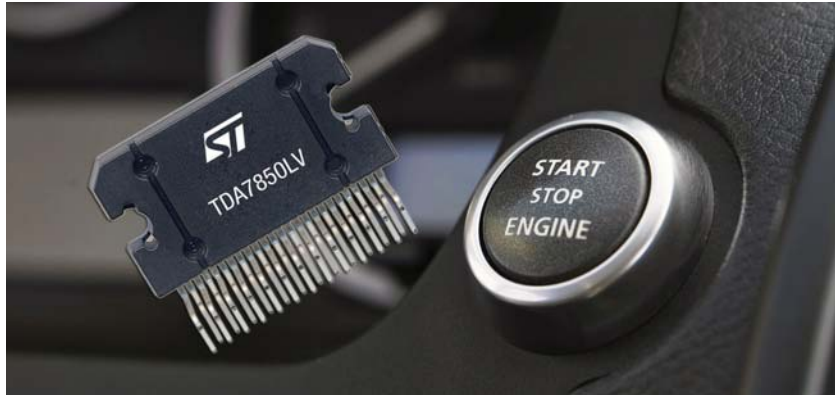
Figure 5 In cars with start/stop, the supply voltage for onboard electrical equipment can fall as low as 6V when a user turns off and restarts the engine. The TDA7850LV audio power amplifier enables in-car-entertainment equipment to operate without interruption during the power-supply dip (courtesy STMicroelectronics).
