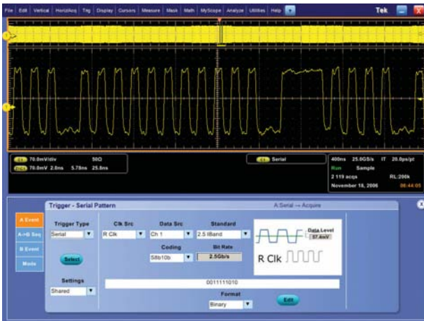
Figure 1 This 5-Gbps PCIe bit stream has 8b/10b encoding triggered on a run-length sequence.
